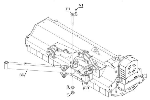
1) Mount the right arm "BD" in the rotation unit "GR" using the pin "P1", the washer "R" and the nut "D". Do not over-tighten it, the arm should rotate freely. Fix the pin in position with its screw "V1";
