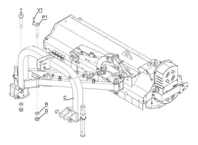
4) Mount the hitch "C" on the right and left arms using the two pins "P1", the two washers "R" and the two nuts "D". Do not over-tighten them, the arms should rotate freely. Fix the pins using the screw "V1"
